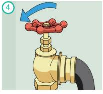
Connect the hose to the fire hydrant and turn the valve to open it.
